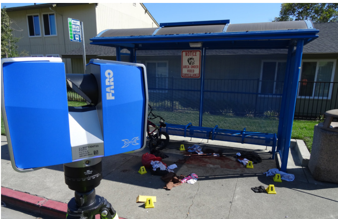
Figure 1. The laser scanner records all the details of a crime scene, like this one, and is much faster than using a total station or manual measurement methods.
