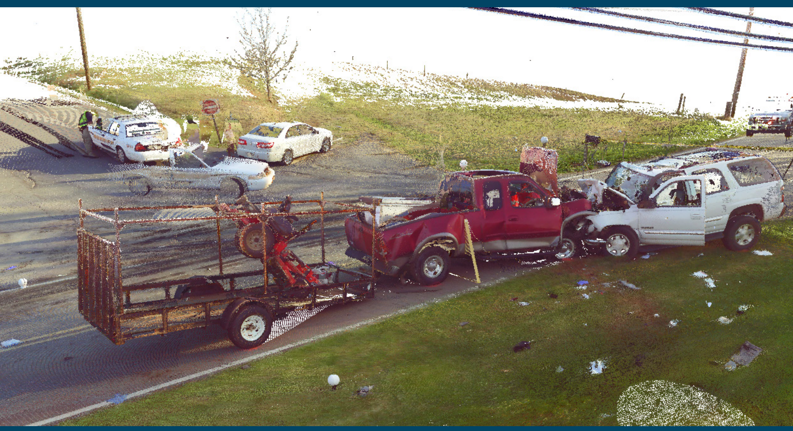
Seven laser scans were used to capture this crash scene. FARO SCENE software was used to register the data from all the scans into a single point cloud.
