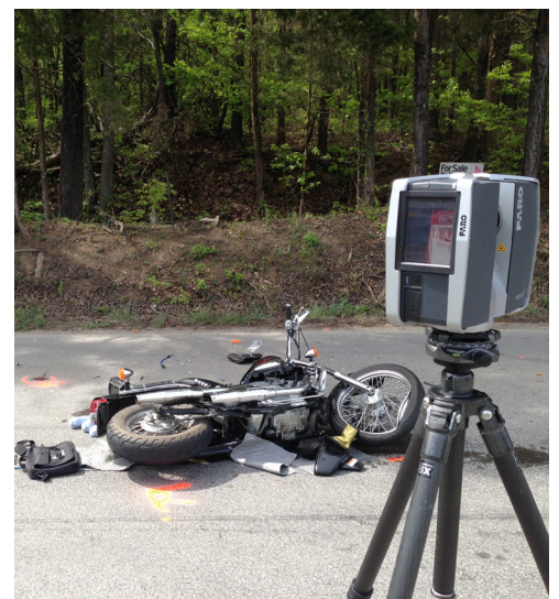
Figure 3. Setting up and starting the scanner quickly, a great deal of data can be captured before any changes have occurred
