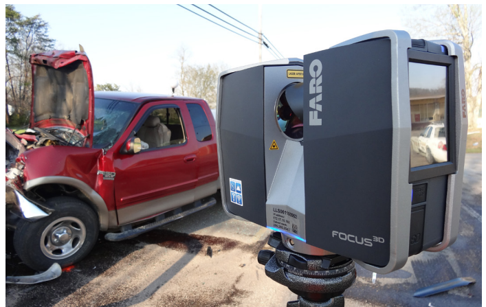
Figure 2. Setting up the scanner at a crash site is quick and easy and eliminates the need for a Total Station.
