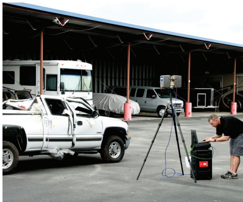
Figure 8. Scanning with the FARO laser scanner
