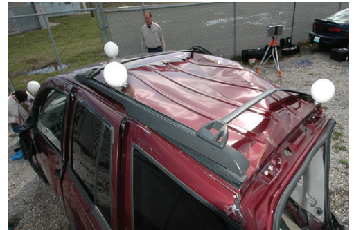
Figure 2. Performing a laser scan of a crashed vehicle.
