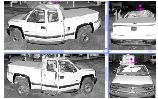
Figure 10. Point cloud of damaged vehicle, full view
