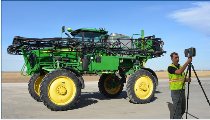
Mark S. Erickson, P.E., sets up the FARO 3D X 130 to scan the farm sprayer that was involved in an incident.
