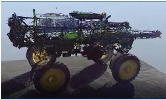
Views of the point cloud of the sprayer, scanned with the FARO 3D X 130 Laser Scanner
