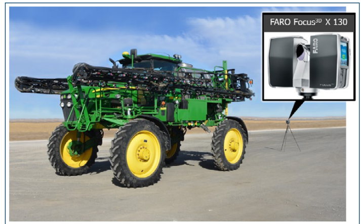
Erickson used the FARO 3D X 130 Laser Scanner to capture an accurate 3D model that could be used to digitally determine the sprayer's field-of-view to the rear.
