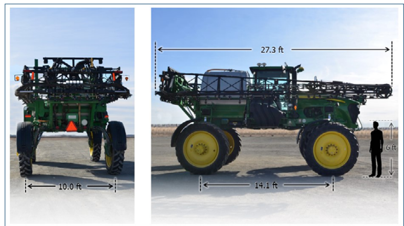
Photographs and overall dimensions of the sprayer.
