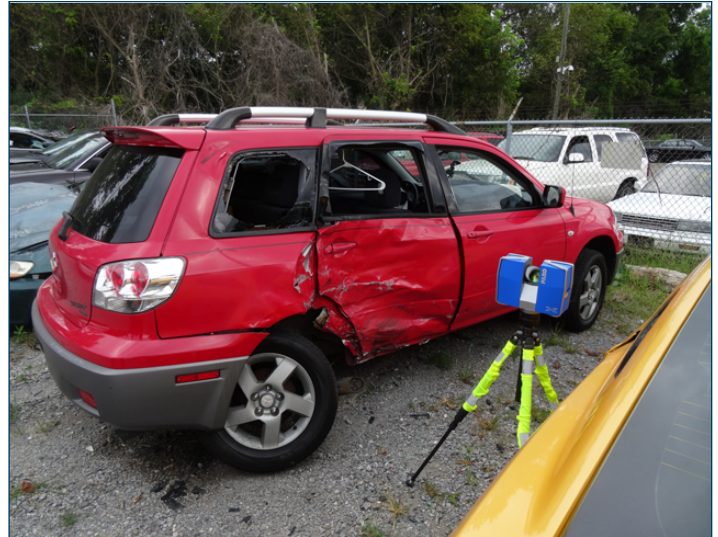
A 3D model of a crashed vehicle can be created by scanning it in the impound lot. That 3D model can be accurately placed in the point cloud of the scene.
