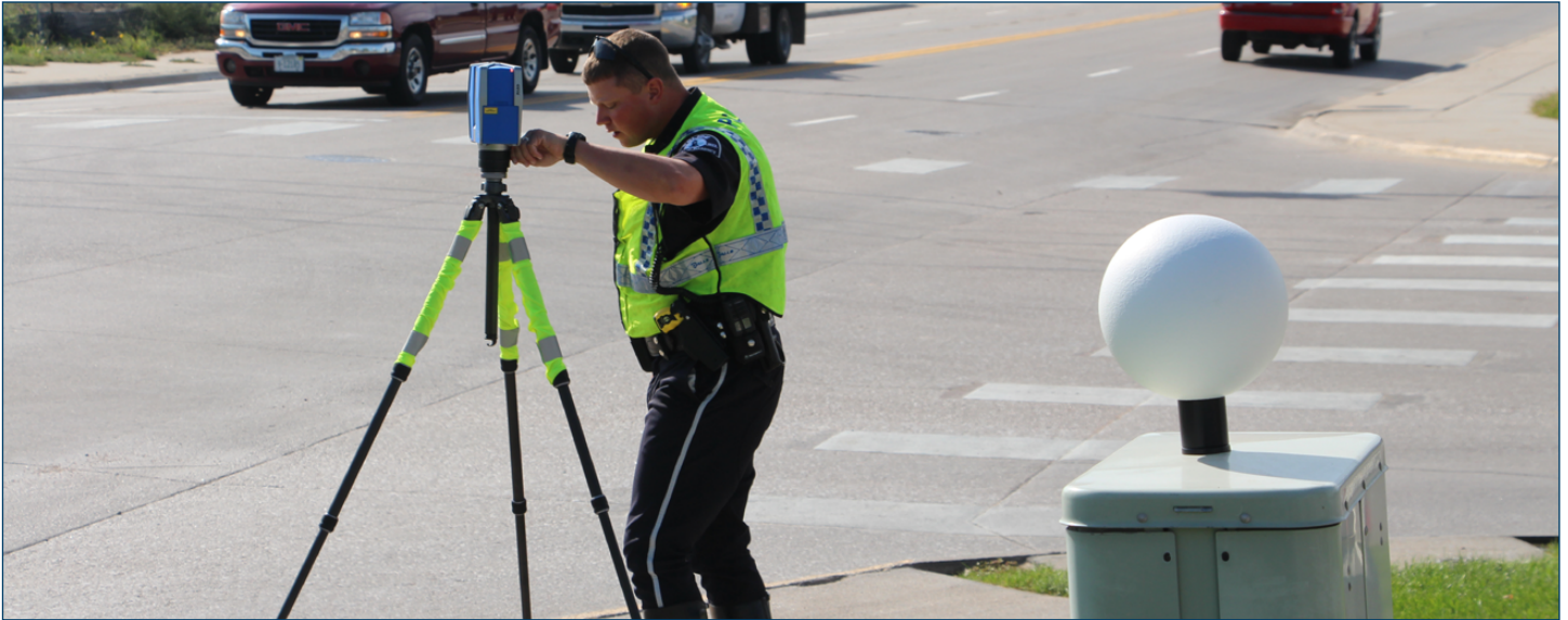
Officer Ryan Ohri, Kearney Police Department, sets up the laser scanner to capture a busy intersection.
