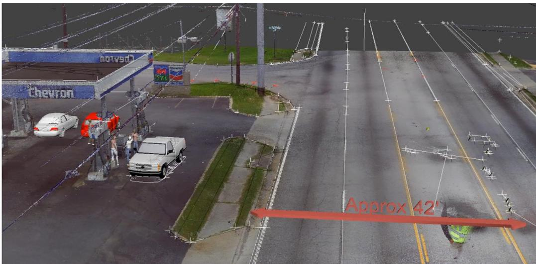
*Figure 1. This image is taken from an animated 3D crime scene created by David Dustin using total station data, surveillance video, and data captured by a FARO 3D Laser Scanner. The arrow shows that, when the victim was hit by a passing car, he was “approximately” 42 feet from the side of the road.*
