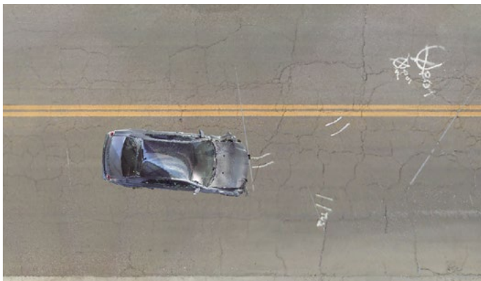
The Chrysler ® was scanned in a salvage yard, and the resulting 3D model was digitally placed into the scene at the position of impact.
