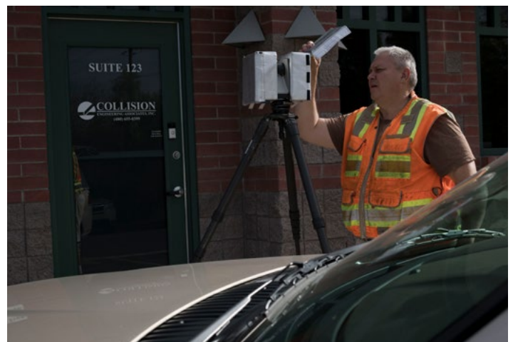
Grimes tested the FARO Focus ® 150 in the Arizona heat, using a special cooling jacket. The jacket is designed to dramatically increase the operating temperature at which the scanner can be used.
