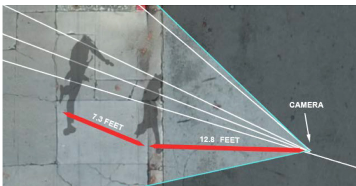
Using the virtual camera, shadows from the camera footage were accurately placed into the point cloud so the distance between the officers and suspect could be measured.
