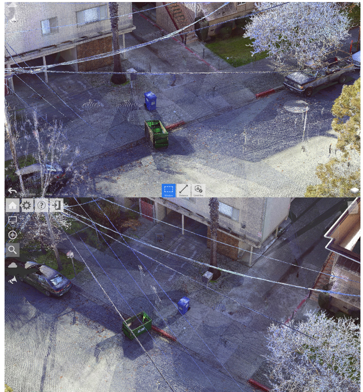
The entire scene was scanned using a FARO Laser Scanner to create a dimensionally accurate, 3D point cloud. The scanned data was used to create a "virtual camera" that could be matched to the point cloud.
